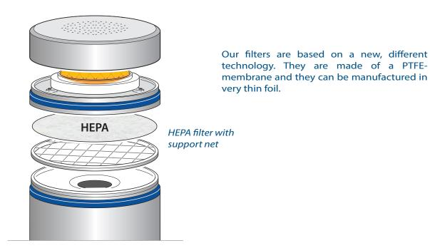
Due to this, it is possible to realize a filter that can be easily installed by the user, a single use filter that can be replaced at the end of each sampling process. A filter of this kind can eliminate any contamination risk maintaining the instrument clean.
